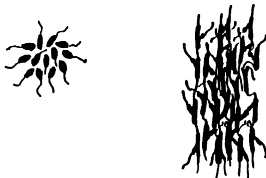
FIGURE 3 Model of the fibrillar packing in the nematic phase. a) in fibrillar direction, b) perpendicular to fibrillar direction.
