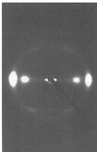
FIGURE 9 X-ray diffraction pattern of wood, X-ray beam perpendicular to the fiber (25°C).
